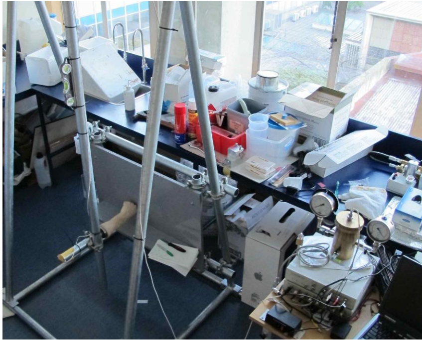
Figure 1. The latest impact machine used to study traumatic fracture in juvenile bone.
