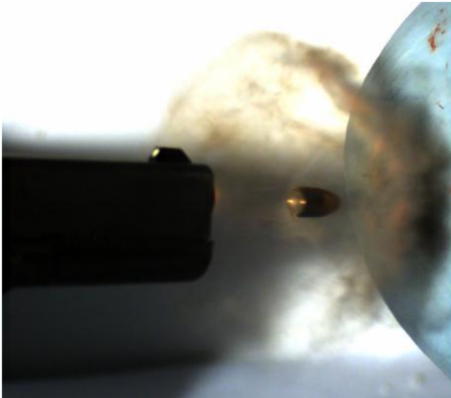
Figure 4 The study of ballistic cranial blood backspatter involves high-speed videography, modeling and biomechanical analysis.
